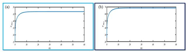
Figure 2: The maximum temperature reached by irradiation of laser on scaffold respected to time for 400mW (A) and at 800mW (B).
