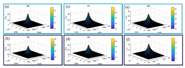
Figure 1: The result of simulating for temperature distribution in the scaffold at t = 2 seconds at 400mW (a) and at 800mW (b), t = 4 seconds at 400mW (c) and at 800mW (d), and t = 10 seconds at 400mW (e) and at 800mW (f)
