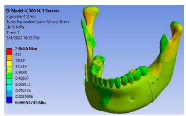
Figure 5: A) The overall tension distribution model of mandible with one miniplate on the right side and three bicortical screws on the left side (Loading force of 300 N on the first molars)
